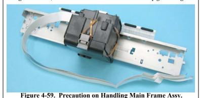
7. Remove the screws (x6) that secure the Main Frame, and remove it while avoiding the LD Roller Shaft so as not to hit the Upper Paper Guide.
