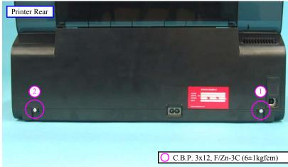
Figure 4-6. Removing Upper Housing (1)
